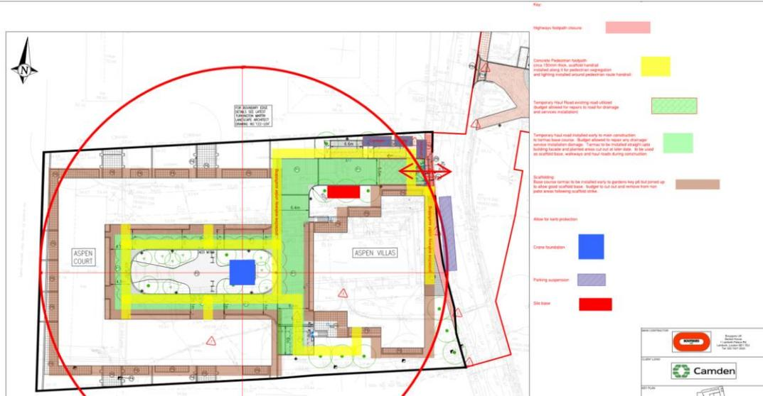
The below site plan shows Grafton Terrace footpath closure highlight in green with hoarding set out into the road to allow use of the footpath on Grafton Terrace to be used as a haul road. The reason this is required is due to the site being surrounded to the back by trees and not being able to use the space to get materials onto site. The footpath will require two crossovers constructing in the areas highlighted below.
