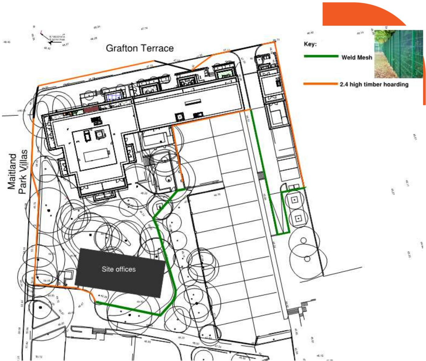
**Figure 6** – Completed hoarding layout around Grafton Terrace. The orange line shows traditional timber hoarding, and the green line represents weld mesh which allows light through and feels less enclosed.
