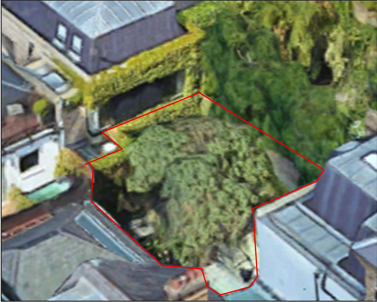
Rear garden 12 years after development (2025) – rear garden area marked in red - basement under 85% of rear garden – pre-development the rear garden was 100% hard paving and had no planting or trees and all the surface water from the hard paving went directly into the public drainage system
